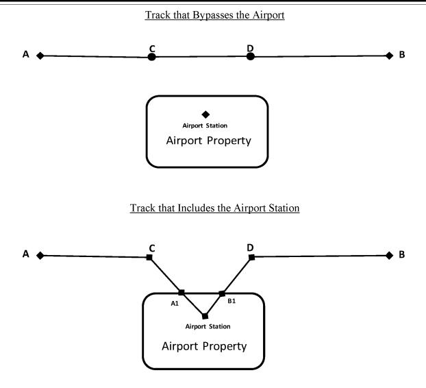
• The approximate incremental cost to serve the airport is the difference between the track cost to serve the airport (C-A1-Station-B1-D) and the cost if the track did not deviate to serve the airport (C-D). This incremental cost represents the costs needed to directly benefit airport passengers and employees. This incremental cost forms the basis of PFC eligibility. However, only that trackage on airport property (A1–Airport Station–B1) is eligible for PFC funding.
